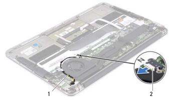
1 routing guides 2 power-adapter connector cable
